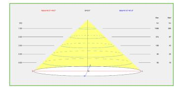
The Illuminance Cone Diagram indicates the maximum illuminance at different distances from the fixture.
