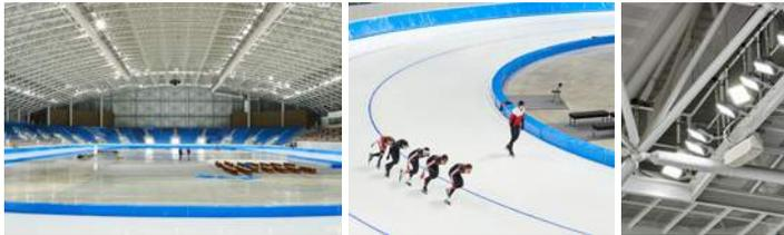
For this project, we installed 452 units of SUFA-A 1.2kW products with a color temperature of 5700K and color rendering of 90 Ra. In addition to a detachable converter, we also included a GeSS lighting control system.
