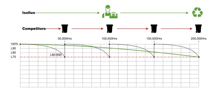
\* HE Chipset L90 Lifetime calculated using 9,000hr independent LM80 photometry report, citing zero failures, using the Energy Star TM-21 protocol. Calculations are based on ambient temperatures of 25°C. With regular maintenance to keep heatsinks and vents clear from blockages. Assumes driver replacement as routine maintenance event at driver replacement at 60,000Hrs. Power tray replacement at schedule to suit customers lux requirements estimated ≥ 100,000 Hrs
